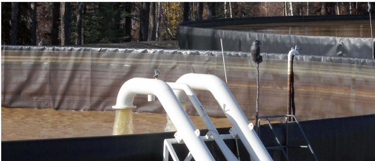
Toxic fracking flow-back fluids into two temporary lined containers alongside an active fracking operation on Talisman’s multi-well pad, 095-I/094-B-01. Note the two fake owls mounted on top of a branch poles, meant to frighten away unsuspecting birds and ducks from an unhappy, toxic fate. Photo by author, September 30, 2010.
