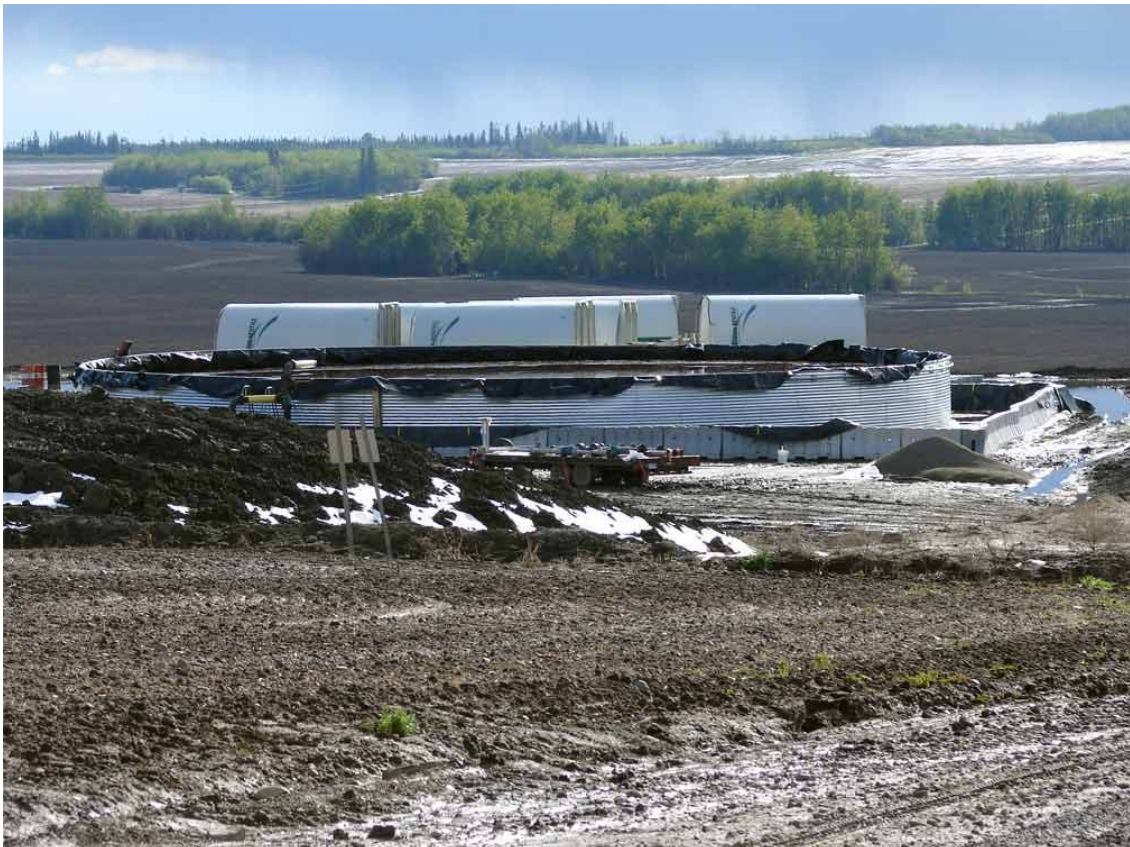
Toxic drilling fluid wastes are temporarily stored in containers on the cleared rectangular pads.
