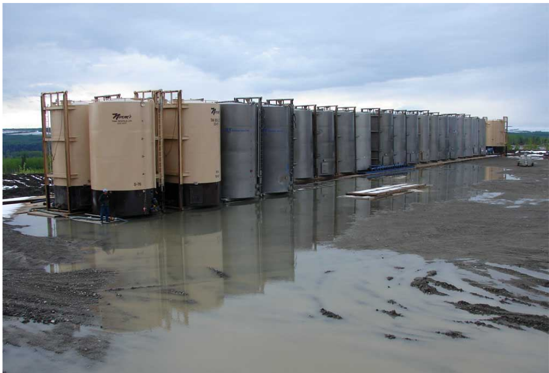
Huge storage tanks for water, with each tank holding a maximum capacity of 64 cubic meters (14,080 imperial gallons), are individually hauled in by trucks and placed on each pad, organized side by side, to be used for the hydraulic fracturing (fracking) procedure.
