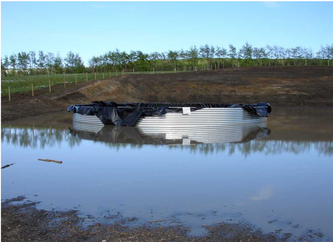
Toxic drilling fluid wastes are temporarily stored in containers on the cleared rectangular pads.
