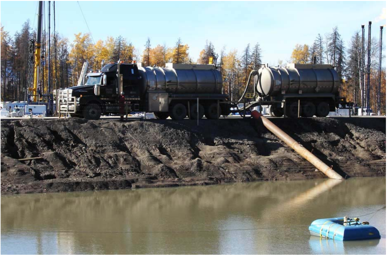
Water truck emptying its fresh water load for Talisman's fracking site.
